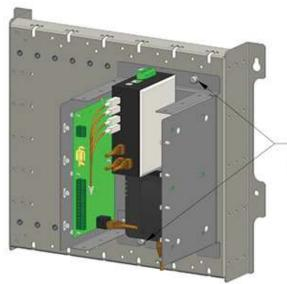
Mount IP Networking Bracket with four M6 x 10 Screws provided with module.
