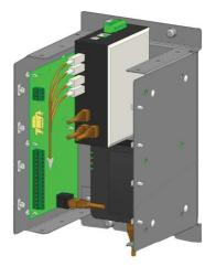
The **QE20-FP2024 Fibre IP Networking Module**, is used alongside the QE20-FP2005 RS485 Network Module to provide a fibre optic cable networking interface for a QE20 system. The fibre network consists of two fibres (TX and RX) wired in a ring around all the QE20 panels on the network. This kit can also be used as a replacement for an existing fibre module.
